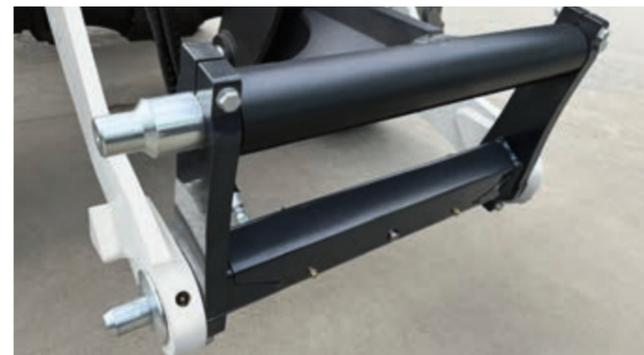
Quicktach coupler (installed as standard)
