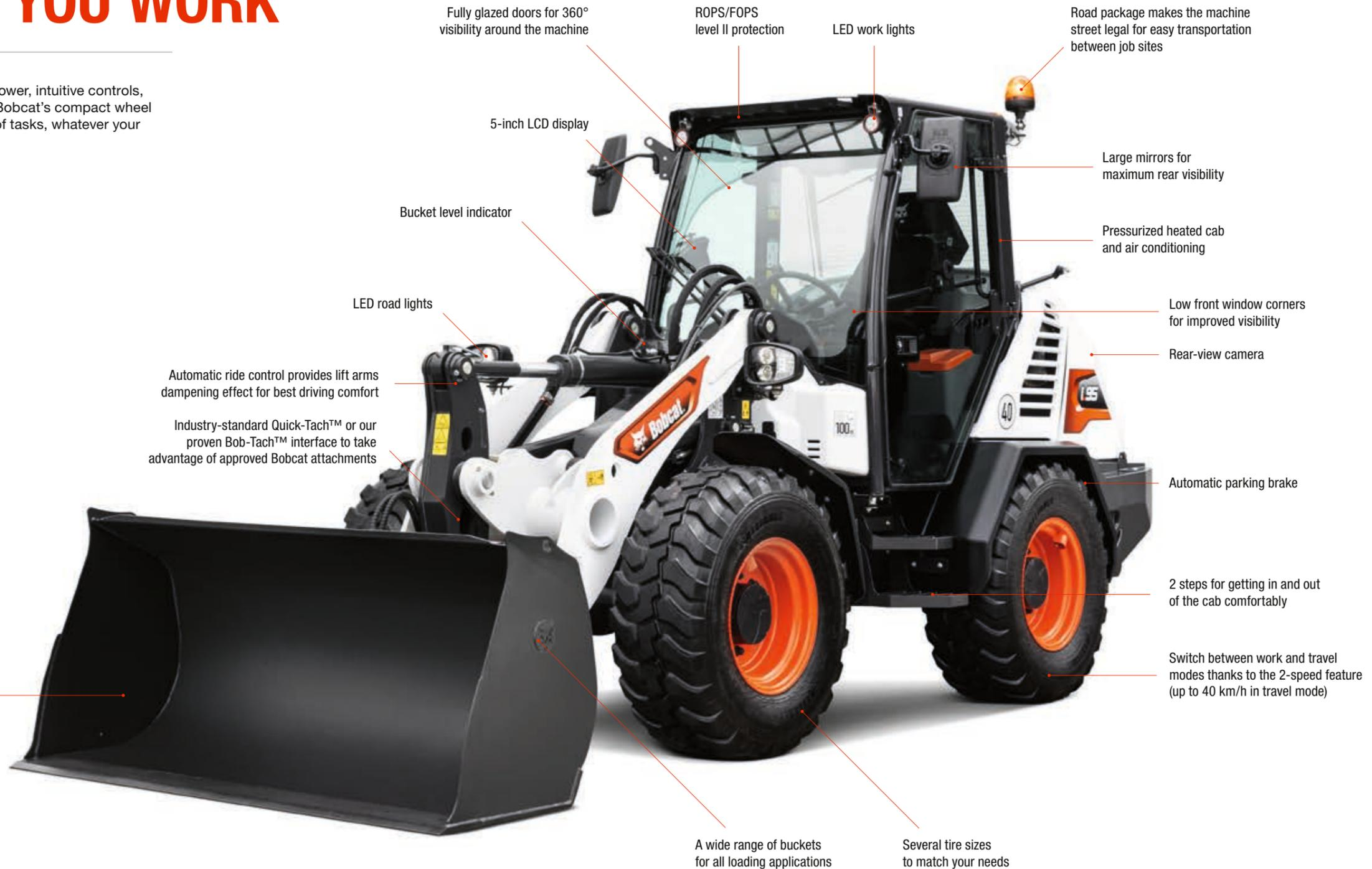
Handle even the most complex attachments thanks to Advanced Attachment Controls, 103 l/min High Flow and a wide selection of attachments.
